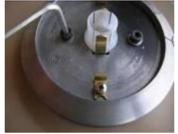
Install the lock case retaining plate over the remaining two studs and screw down the two brass pillars. If need be loosen the pillars to ensure that the flats point towards each other.
