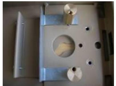
It may be necessary to trim the front cut out in the front of the lock case cover. If it is hinged it may be trimmed using tin snips or a small hacksaw and file. Alternatively the cover may be removed if required.
